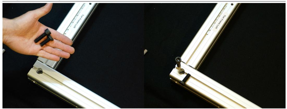
In the bag with the nuts and bolts for this part of the assembly, you shall find two types of the same 10mm bolt. There should be a normal bolt and one with a shorter head and length. Each corner requires 1 of each type.
