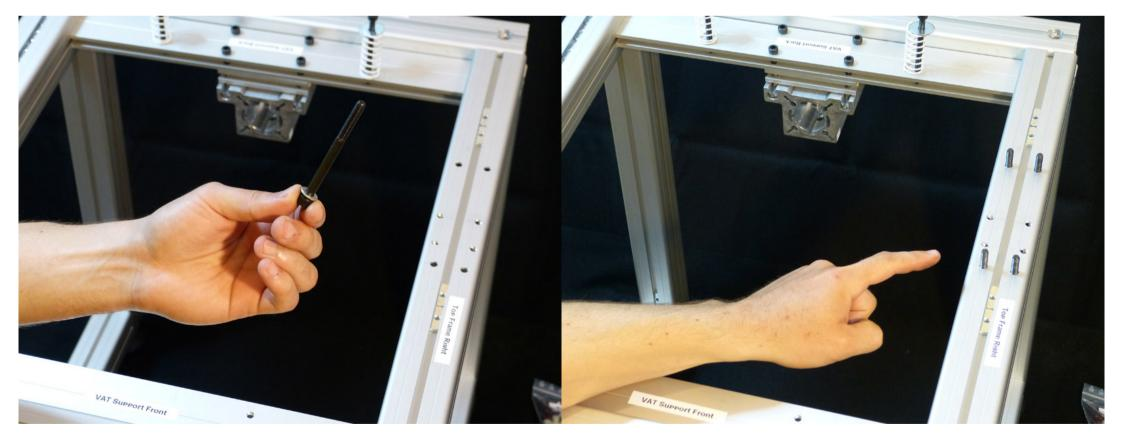
Don't forget to place a washer on these bolts, they spread the load more evenly and help keep the structure strong. Note how the Sliding Nuts on the main frame have been separated in pairs on each side. Do this now for later assembly.
