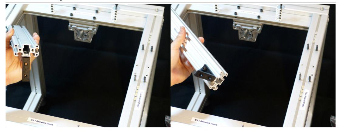
Bolt the corner as shown. Note that if you already see where this is going, the corner should have its edged wall looking outwards from important and although the alignment shall be accurate, make it the machine (this is for esthetics and doesn't matter mechanically)
