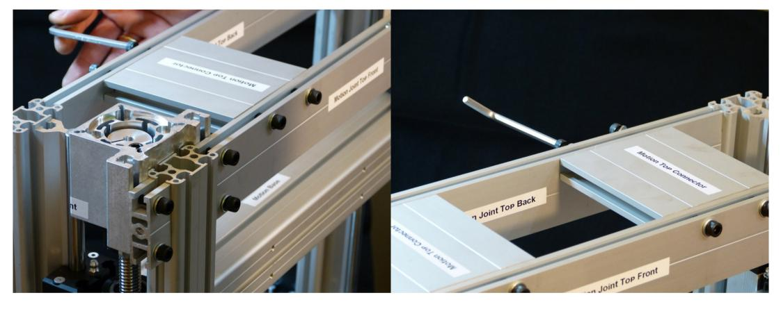
Next, tighten the back side of the connector. Make sure that it is Repeat the process for the other side of the assembly, tightening nice and tight so that the frame is as rigid as it can be.
