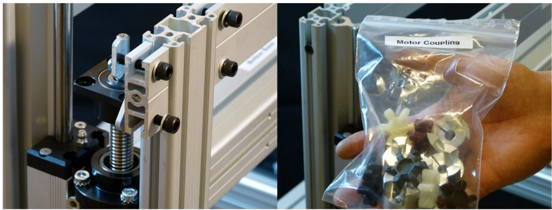
Use the Oval Sliding nuts and 4 bolts with their washers as shown Take the Motor Coupling bag and prepare to assemble it as shown on the image above. They shall hold the motor mount in place on the image above.
