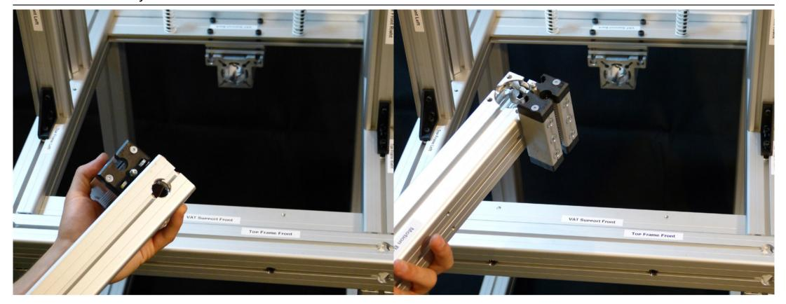
Slide the Slider block through the Oval nuts and center it on the Tighten the bolts and you should have a result like shown on the assembly. The centering is not very crucial and is only for estheticsimage above. Note the orientation of everything in the assembly at but make it as center as you can by eye. this point.
