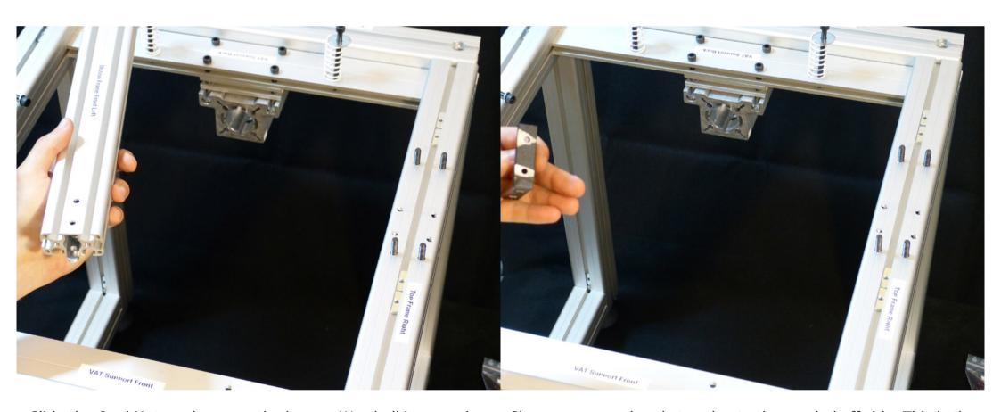
Slide the Oval Nut as shown on the image. We shall be securing the corner brackets with them later on.
