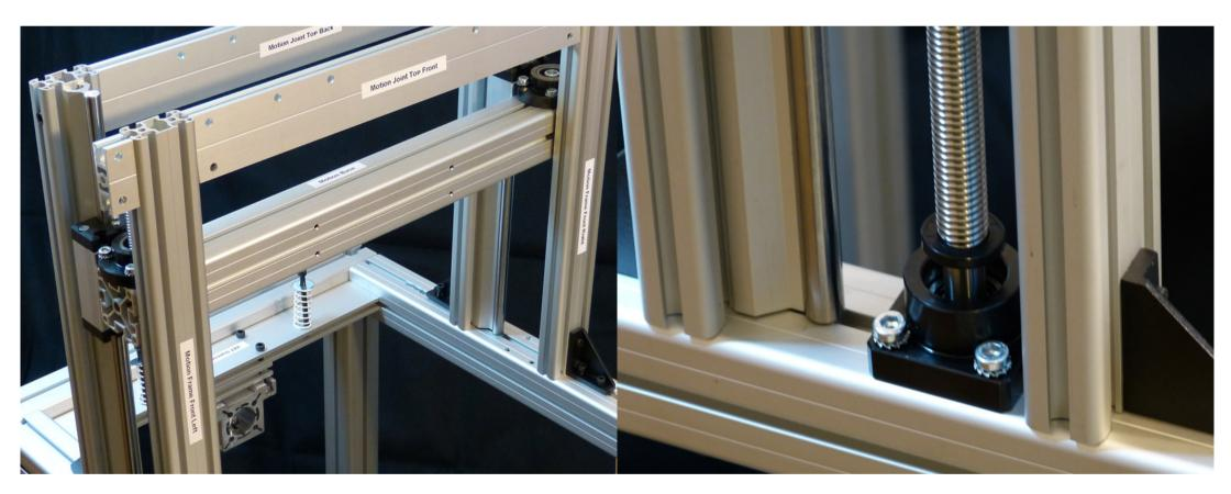
Push it down a bit until the first spindle touches the support bearing.
