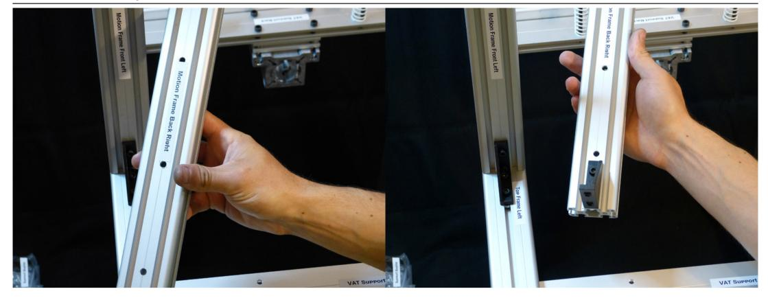
Select the Back frame part and do the same process with it, attaching it to the back side of the main frame.
