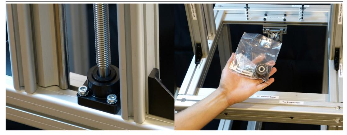
NOTE that the rubber seal should be TOUCHING the start of the spindle and NOT have any space from the bearing left, meaning that the spacing as shown on the image above should NOT be left like that but pushed all the way in.
