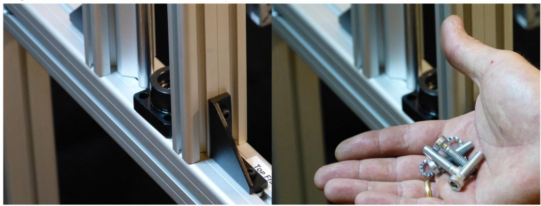
Place the support bearing on the frame as shown. We shall bolt it Take the 6mm bolts and their washers (included in the bag) and on but not tight, so that there is play and room to adjust it.
