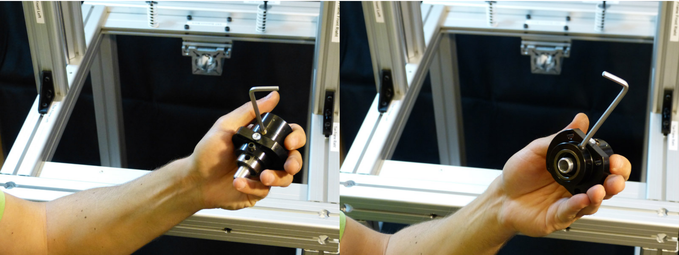
Slide the nut into the housing. Note the hole on the nut it self, it should align with the outer bolt ans it shall secure it in place. Push the spindle nut all the way in and tighten the headless bolt so that it aligns the assembly and centers it as needed.
