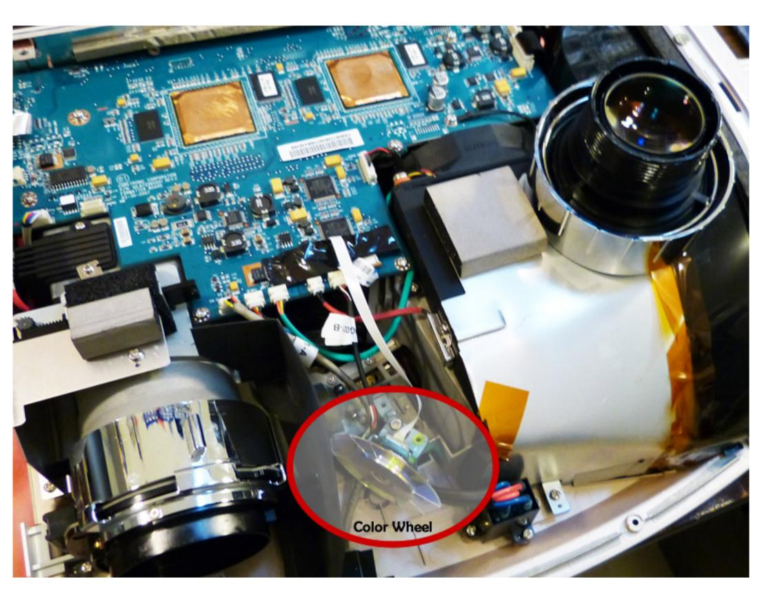
In cases where there is enough space within the projector, you can simply place it within the enclosure, removing it from the light path. In other cases you shall have to brake off the glass from the wheel motor. Unfortunately you cannot just unplug the motor from the projector since it shall most likely cause an Error within the projector software and not make it function at all.
