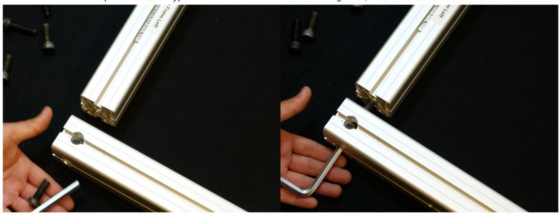
First we take the shorter bolts, to connect each side of the Top Frame. It is important that this bolt goes in first.
