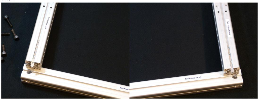
Before we begin bolting everything together, we need to add the four (4) Oval Slide nuts to the slots as shown. These have to go to the Left and Right parts of the frame (on the top slot). These nuts have a 5mm thread (important to note and not confuse with the 6mm thread) and shall hold the motion framing later on.
