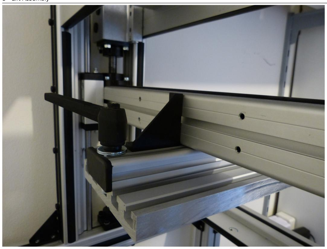
In the image above you can see how the Small Lift is mounted on the Lift Arm. The screw holes should already be on the arm so all you need to do is mount the lift as shown. If you purchased Both Large and Small lifts then use the bolts provided from ether assembly.
